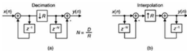
Fig. 9 Single-stage CIC filters implementations: (a) For decimation (b) For interpolation
