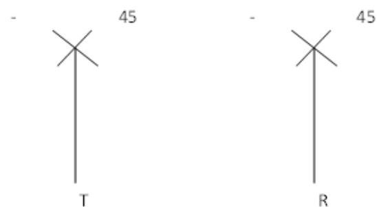
Figure 2.1. Schematic of dual-polarized slanted antenna setup both at the transmitter ( T_X ) and the receiver ( R_X ) side.
