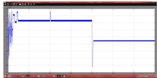
Fig.10.4. Reactive power consumed by the loads
