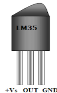
Figure:4 Temperature sensor
