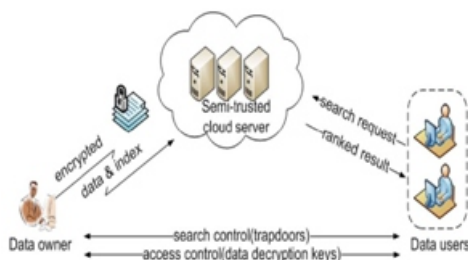
Fig. 1. Architecture of the search over encrypted cloud data
