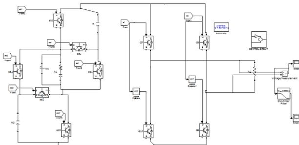
Fig. 5 Matlab/Simulink Model of Proposed Single Phase Series/Parallel Converter.
