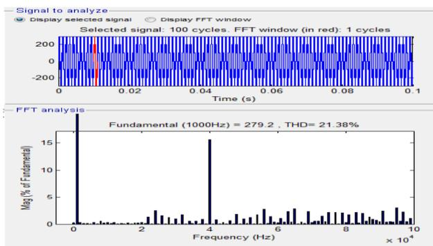
Fig. 7 FFT Analysis of Output Voltage without Filter of Proposed Series/Parallel Converter.
