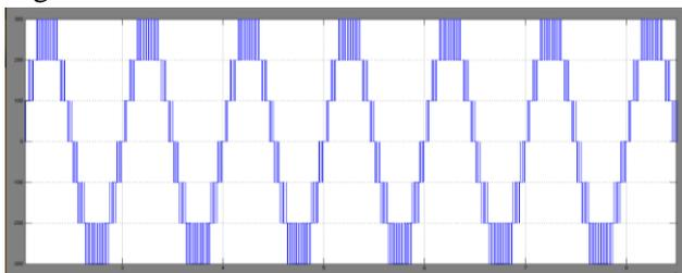
Fig. 6 Seven Level Output Voltage.
