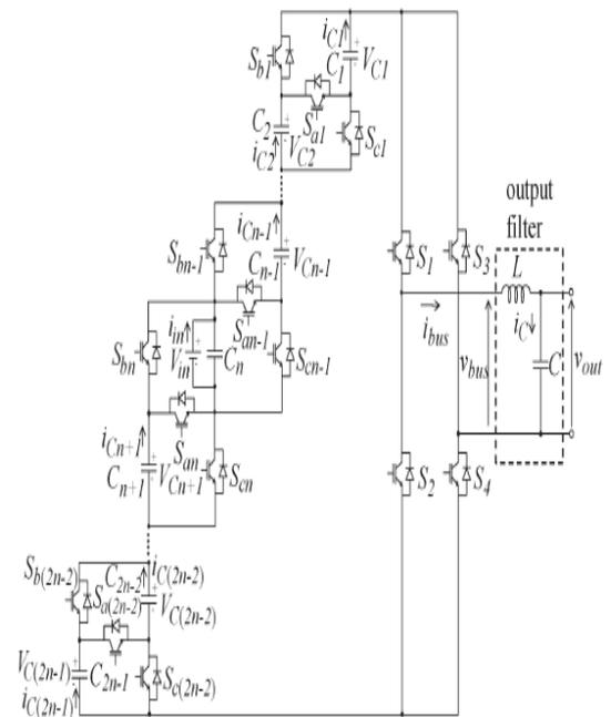
Fig.1. Circuit topology of the switched-capacitor inverter using series/parallel conversion.
