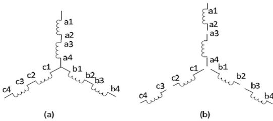
Fig. 4 Induction Motor stator winding: (a) General arrangement (b) Arrangement for the proposed inverter
