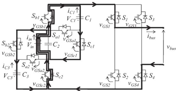
(b) All capacitors are connected in Parallel.
