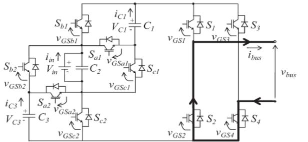
(a) The current  $i_{bus}$  does not flow in the capacitors  $C_k$ ,
