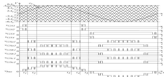
Fig.3. Modulation method of the proposed inverter ( $n = 2$ ).
