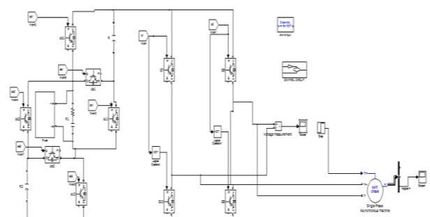
Fig. 9. Matlab/Simulink Model of Proposed Series/Parallel Converter Applied to Single phase IM Drive.
