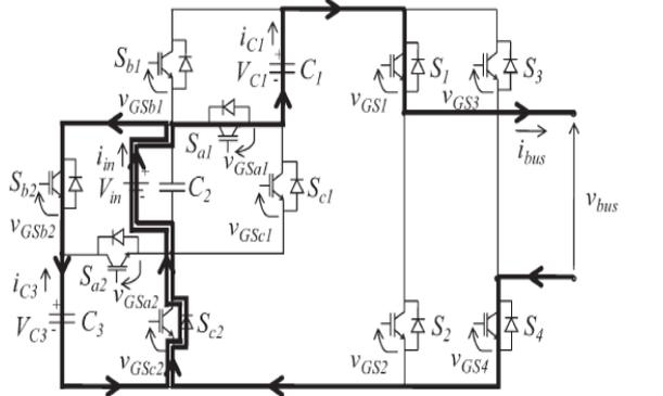
(c) The capacitor  $C1$  is connected in series and the capacitor  $C3$  is connected in parallel.
