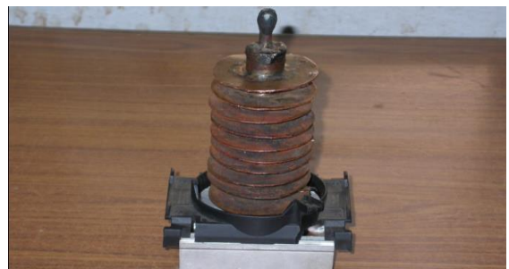
Fig: 4.11 Photo of the Heat Pipe used for the Experiment Base plate, circular fin, Pipe (copper) & Lid
