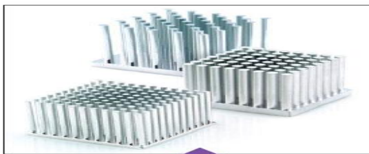
Fig. 2. Heat sinks with three different pin configurations for: low air speed (top), moderate air speed (middle) and high air speed (bottom).
