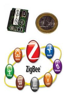
ZigBee module. The €1 coin, shown for size reference, is about 23 mm (0.9 inch) in diameter. ZigBee is a specification for a suite of high level communication protocols using small, low-power digital radios based on the IEEE 802.15.4-2003 standard for wireless personal area networks (WPANs), such as wireless headphones connecting with cell phones via short-range radio.
