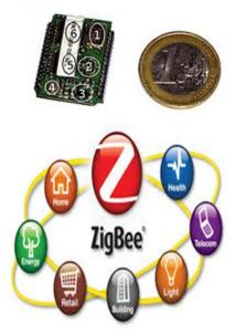
ZigBee module. The €1 coin, shown for size reference, is about 23 mm (0.9 inch) in diameter. ZigBee is a specification for a suite of high level communication protocols using small, low-power digital radios based on the IEEE 802.15.4-2003standard for wireless personal area networks (WPANs), such as wireless headphones connecting with cell phones via short-range radio.
