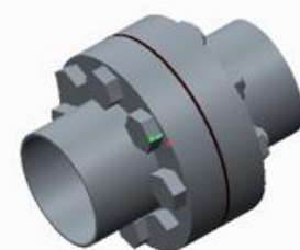
Fig-2. Assembled Flange joint
