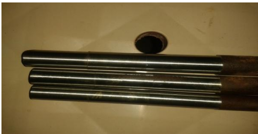
Prepared Work pieces after cylindrical Grinding Process
