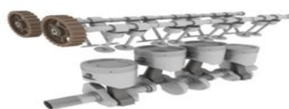
Inline four engine piston arrangement
