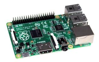
The Raspberry Pi has a Broadcom BCM2835 system on a chip (SoC), which includes an ARM1176JZF-S 700 MHz processor (The firmware includes a number of "Turbo" modes so that the user can attempt over clocking, up to 1 GHz, without affecting the warranty), VideoCore IV GPU, and was originally shipped with 256 megabytes of RAM, later upgraded to 512 MB. It does not include a built-in hard disk or solid-state drive, but uses an SD card for booting and long-term storage
