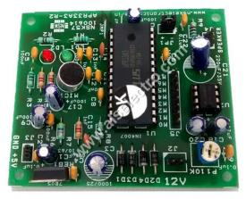
The aPR33A series are powerful audio processor along with high performance audio analog-to-digital converters (ADCs) and digital-to-analog converters (DACs). The aPR33A series are a fully integrated solution offering high performance and unparalleled integration with analog input, digital processing and analog output functionality.
