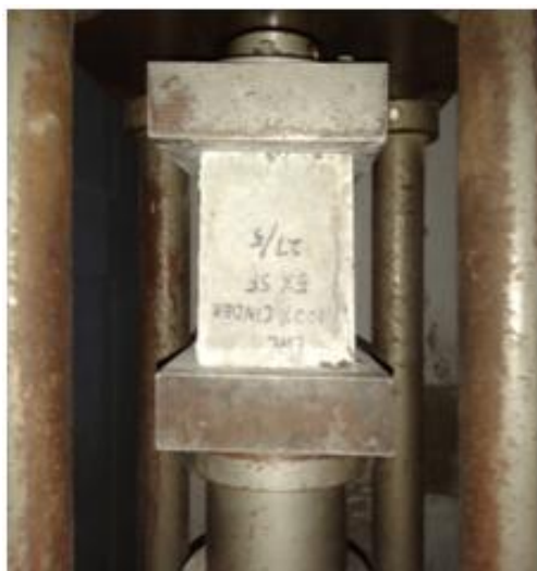
Testing of cube FIGURE
