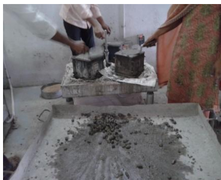
Casting of cubes with vibrator
