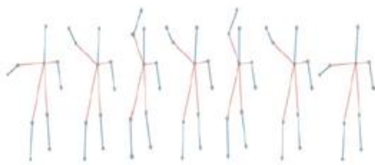
Fig. 3. Posture sequence from one repetition of the “high arm wave” gesture.
