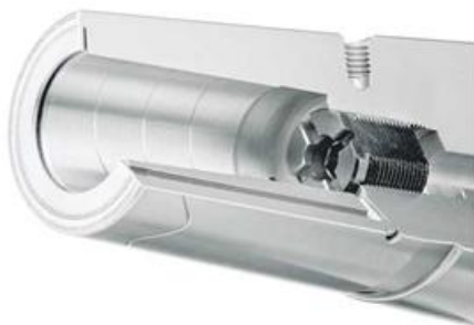
With the Haimer Cool Flash System, there is a disc at the end of the shrink fit chuck that releases a narrow circumferential gap in the direction of the tool. This allows the coolant to wrap itself around the tool like a jacket.
