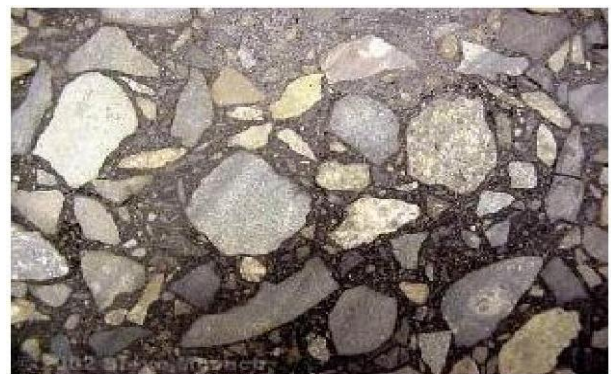
Fig. 2.1 Dense graded HMA surface
