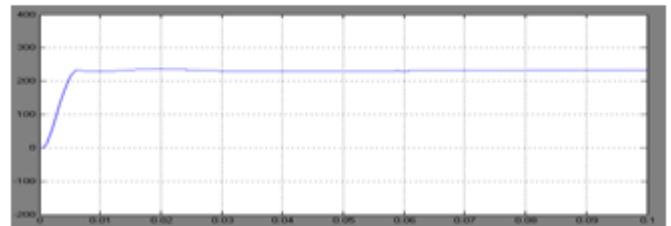
Figure 14: Converter DC voltage under operating condition using pwm
