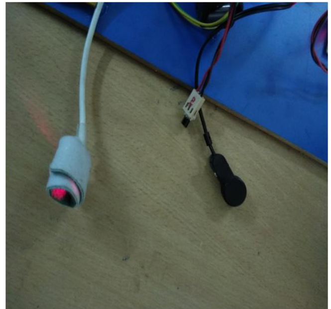
Fig 5.3: Pulse rate, temperature and SPO2 Sensors of proposed system
