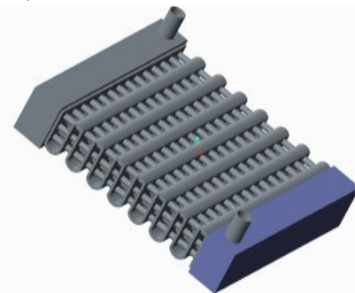
Fig. 1.3 3D Model of the Radiator
