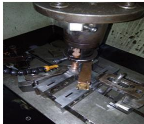
Fig – Machining of work piece using Hexagonal electrode
