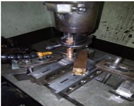
Fig – Machining of work piece using round electrode
