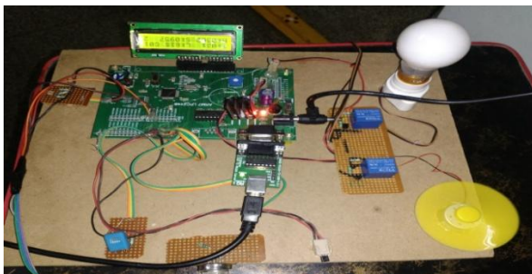
Fig 8 Kit prototype of sensor node-2 giving toggle to the fan when command=2
