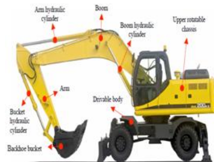
Fig 1.2 Main parts of excavator from website ref (15)
