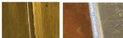
Figure 2: Brass, as well as mixed copper / aluminum joints can be friction stir welded.
