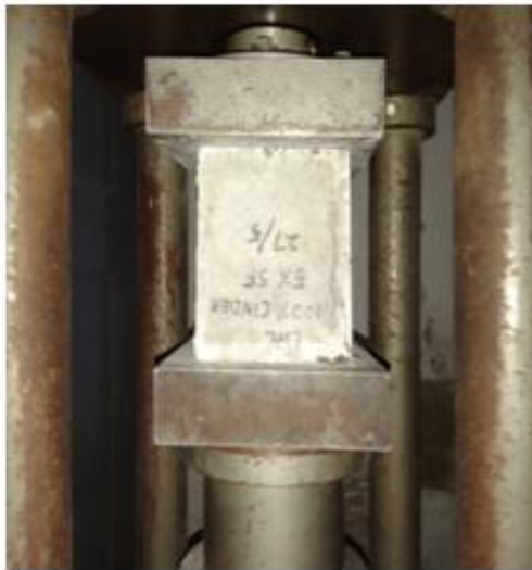
Testing of cube FIGURE
