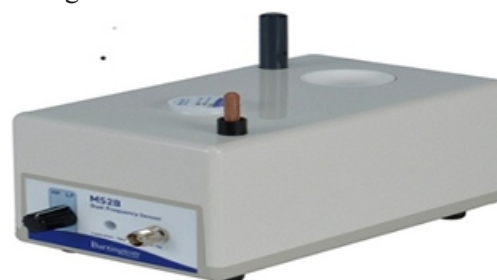
Fig .4: Magnetic Susceptibility System - BARTINGTON MS 2B dual frequency sensor.
