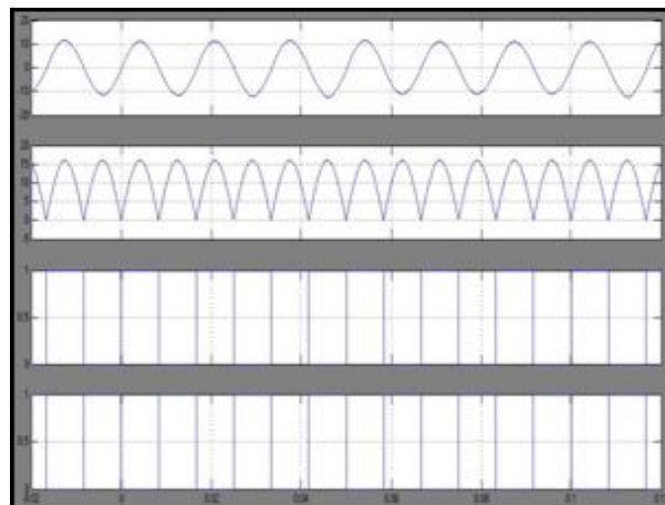
Figure 8: Simulation results of Output current of the full-bridge inverter, Input current of the full bridge inverter, Driver signal of S4, Driver signal of S5.
