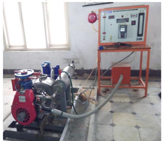
Fig.7.1: Variable Compression Ratio SI Engine – Experimental Setup
