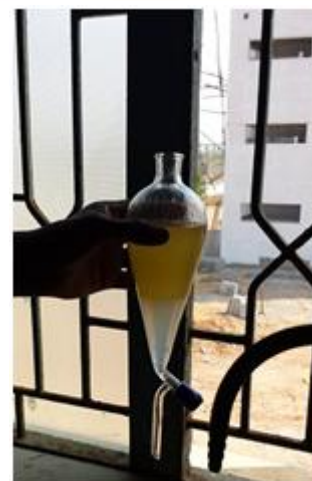
Fig: Experimental Setup for production of Palm oil as Biodiesel.
