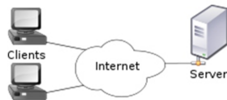
Fig: A computer network diagram of clients communicating with a server via the Internet.
