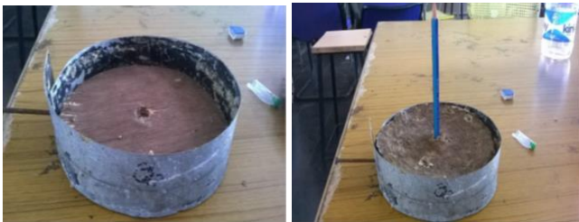
Fig.4.2. The above figure shows the disc pattern of sample with an outer diameter of 150mm and thickness of 10mm with a hole of 13mm diameter for fixing of bolt.
