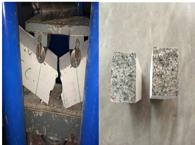
Fig: 5 Flexural beam specimens under test.
