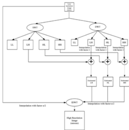
Fig3. Proposed block diagram of DUWT with interpolation method
