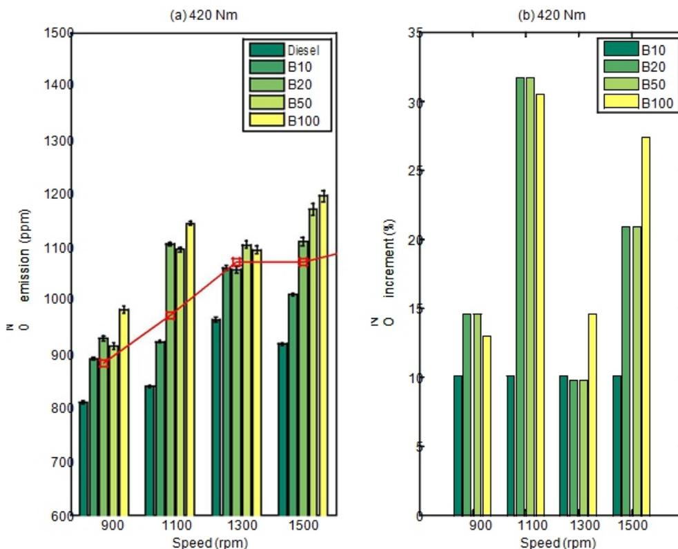
Figure 8. (a) Variation of NOx emissions with engine speed for CI engine running with biodiesel blends at a load of 420 Nm; (b) NOx emission reductions due to biodiesel blends (B10, B20, B50, B100) comparing with diesel at 420 Nm.
