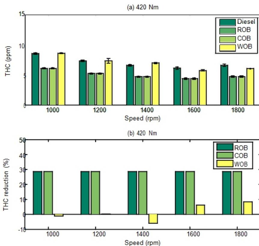
**Figure 5. (a) Variation of THC emission of CI engine running with ROB, COB, WOB and diesel at a load of 420 Nm; (b) THC emission reductions in percentage comparing biodiesel (ROB, COB, WOB) with diesel at 420 Nm.**
