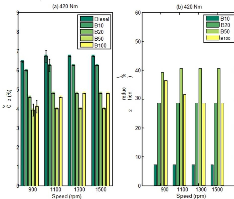
Figure 7. (a) Variation of CO<sub>2</sub> emissions with engine speed for CI engine running with biodiesel blends at a load of 420Nm; (b) CO<sub>2</sub> emission reductions due to biodiesel blends (B10, B20, B50, B100) comparing with diesel at 420 Nm.
