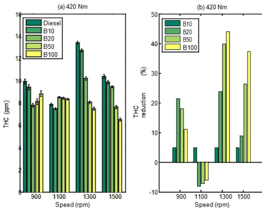
Figure 9.(a) Variation of THC emissions with engine speed for CI engine running with biodiesel blends at a load of 420 Nm; (b) THC emission reductions due to biodiesel blends (B10, B20, B50, B100) comparing with diesel at 420 Nm.
