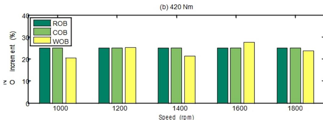
**Figure 4. (a) Variation of NOx emission of CI engine running with ROB, COB, WOB and diesel at a load of 420 Nm; (b) NOx emission reductions in percentage comparing biodiesel (ROB, COB, WOB) with diesel at 420 Nm.**
