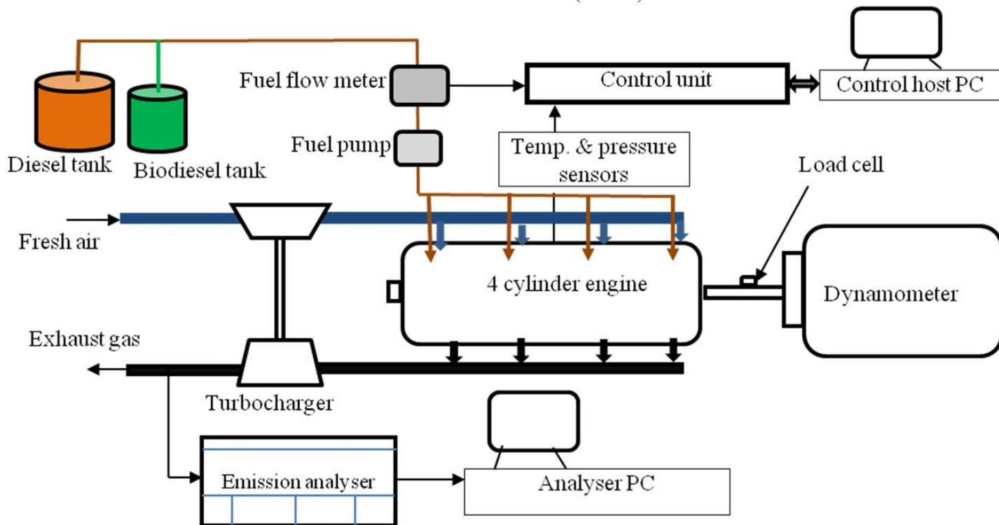
**Figure 4. Engine test facilities layout [46].**
