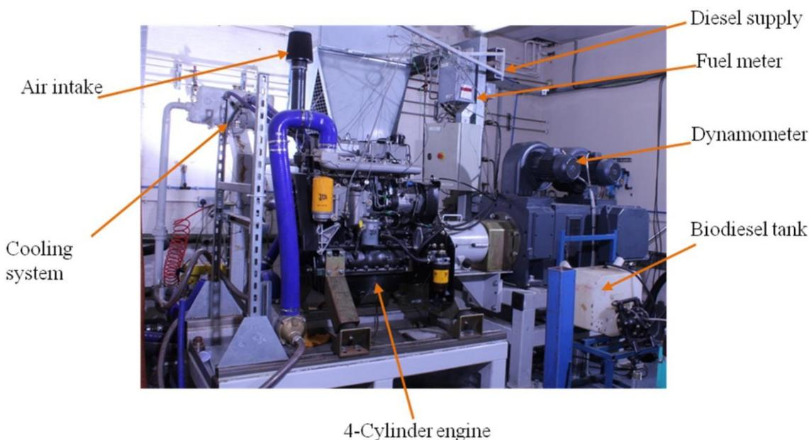
**Figure 3. Experimental engine facilities.**
