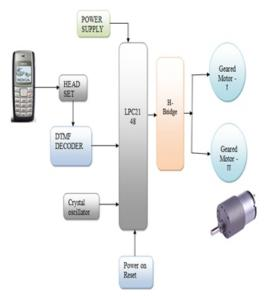
The LPC2148 are based on a 16/32 bit ARM7TDMI-S<sup>TM</sup> CPU with real-time emulation and embedded trace support, together with 128/512 kilobytes of embedded high speed flash memory.
