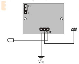
The Passive Infrared Sensor (PIR) sensor module is used for motion detection. It can be used as motion detector for security systems or robotics. It works form 3.3V to 5V DC and gives TTL output which can be directly given to microcontroller or to relay through a transistor.
