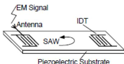
Fig. 2. Schematic of a passive SAW sensor
