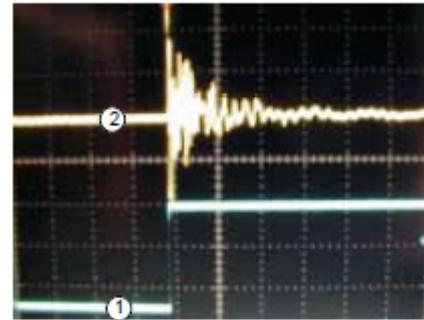
Fig. 9. A transducer driven by a step function voltage, with the time base 100  $\mu$ s/div. 1) An electrical step function, 2 V/div. 2) Received ultrasonic pulse, 20 mV/div.
