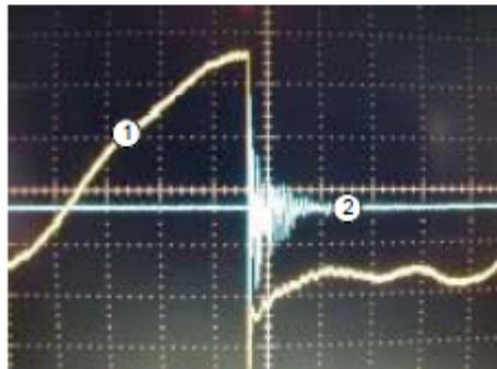
Fig. 12. Ultrasonic transmitter excited by the step voltage, with time base 20  $\mu$ s/div. 1) The voltage measured between the two faces of the stack, 100 V/div. 2) The voltage measured at the output of AE sensor, 2 V/div.
