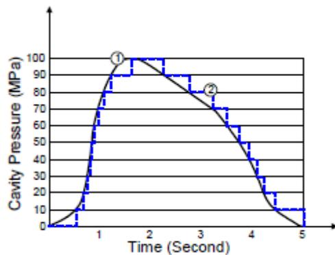
Fig. 3. The concept of digitized pressure measurement
