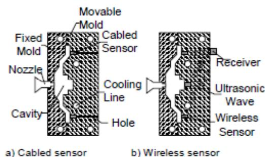
Fig. 1. Schematics of cabled sensor and wireless sensor installed in a mold
