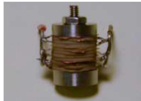
Fig. 10. A ten-piezoelectric ring stack
