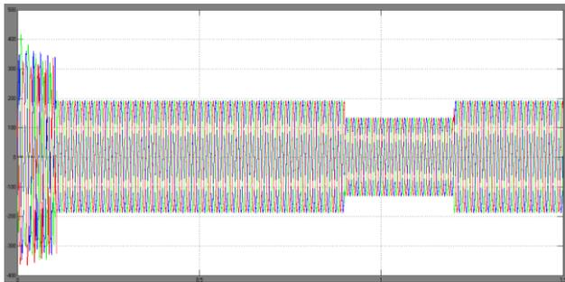
Fig.14. Simulation results for Source Voltage During Sag.
