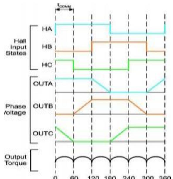
Fig.6. Hall signals & Stator voltages.
