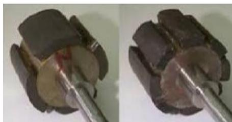
Fig.5. BLDC motor Rotor construction.
