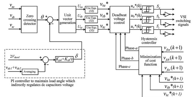
Fig.3 Overall block diagram of the controller to control DSTATCOM in a distribution system.
