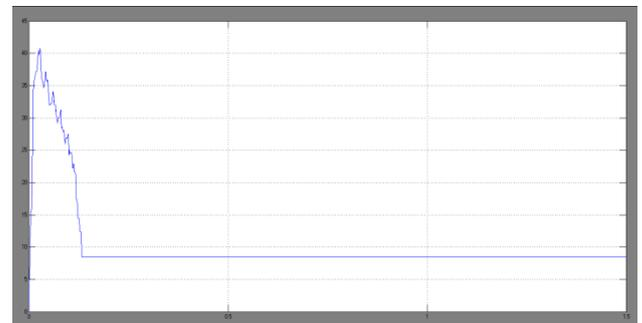
Fig.12. Phase- compensator RMS currents.
