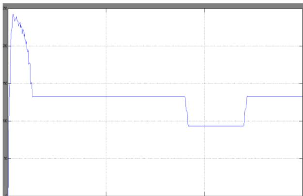
Fig.15. simulation result for RMS value of source voltage during sag
