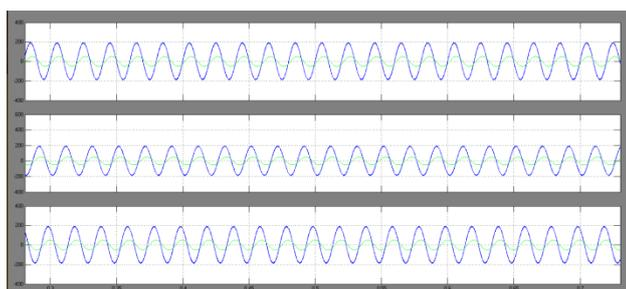
Fig.10. Terminal voltages and source currents using the traditional method. (a) Phase-A. (b) Phase-B. (c) Phase-C.
