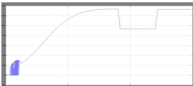
Fig.16.Simulation results for dc link voltage.
