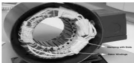
Fig.4. BLDC motor stator construction
