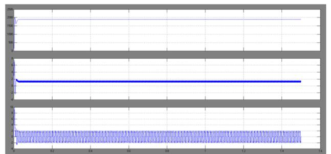
Fig.20.speed, torque and armature current of BLDC drive.
