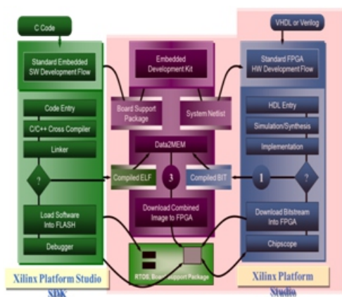
Fig7: Embedded Development Kit Design Flow
