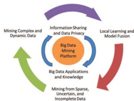
Fig.2. A Big Data processing framework: The research challenges form a three tier structure and center around the “Big Data mining platform” (Tier I), which focuses on low-level data accessing and computing. Challenges on information sharing and privacy, and Big Data application domains and knowledge form Tier II, which concentrates on high-level semantics, application domain knowledge, and user privacy issues. The outmost circle shows Tier III challenges on actual mining algorithms.
