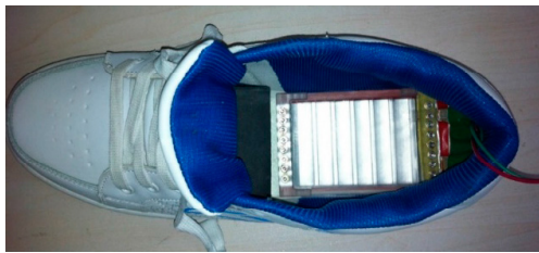
Figure 6. (a) Prototype 1 with an 8-layer PVDF film was mounted on the inner sole and gathered energy under the heel.
