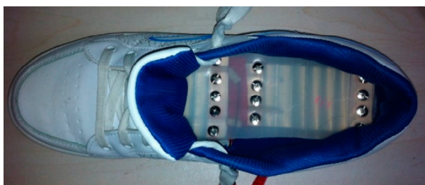
(b) Prototype 2 with two 8-layer PVDF films was used as a normal insole in a shoe.
