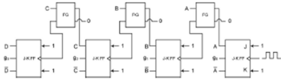
Fig. 5. Proposed design of 4-bit reversible sequence counter.
