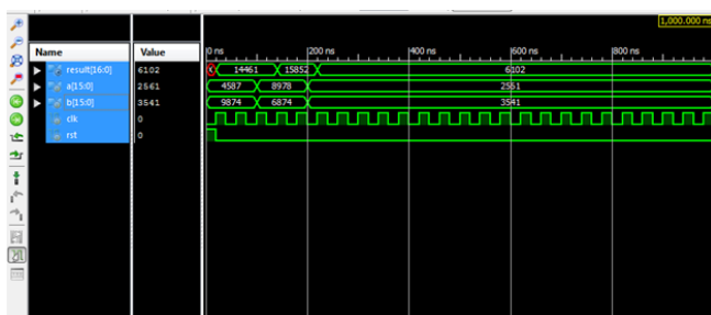
Fig12: Simulation output waveform of 16bit-BK-BEC Carry select adder
