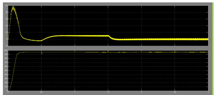
Fig.3.(b). Simulation results under SMC+ESMDO: torque and speed
