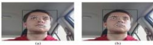
Fig 3 (a) Mean landmarks, x_0 , initialized using the face detector. Black outline indicates face detector.
