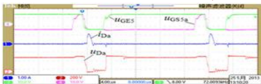
Fig. 12. Experimental waveforms of the auxiliary switch S5a ( u_{GE5} and u_{GS5a} : 10 V/div, u_{S5a} : 100 V/div, i_{S5a} : 2 A/div, and time: 4 \mu s/div).
