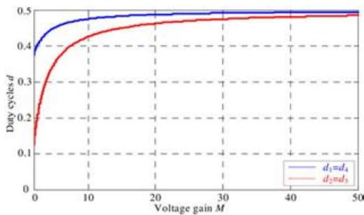
Fig.6. Duty cycles curves versus voltage gain.
