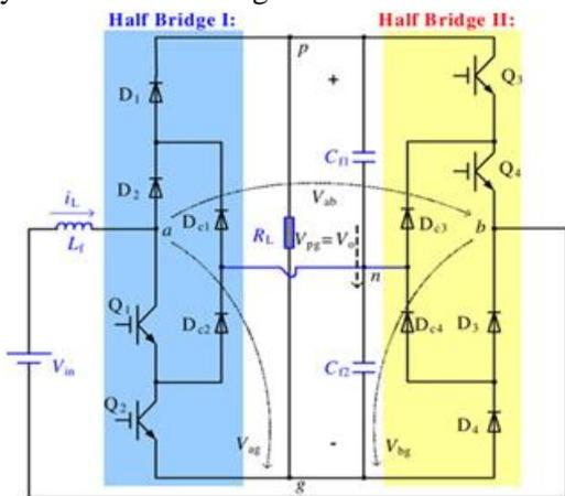
Fig. 4. Proposed hybrid boost three-level dc-dc converter.
