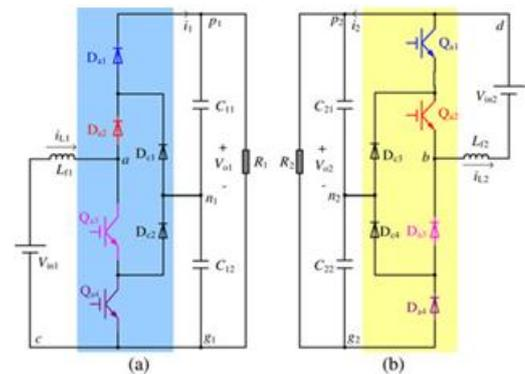
**Fig. 2. Two deduced boost three-level dc-dc converters.**
