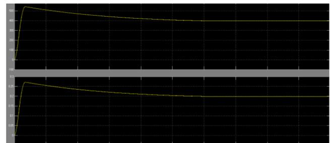
Fig. 9. Output dc voltages and inductor current under the load step change from  $720 \Omega$  to  $360 \Omega$ .
