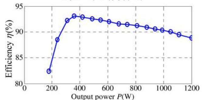
Fig. 10. Measured efficiency of the proposed converter.
