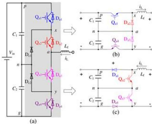
**Fig. 1. Single-phase diode-clamped three-level inverter and two classical three-level dc-dc converters.**
