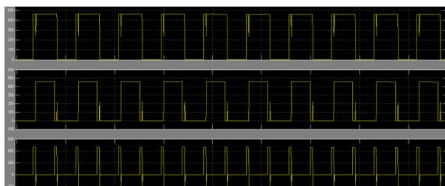
Fig. 8. Output three-level voltages of the converter.
