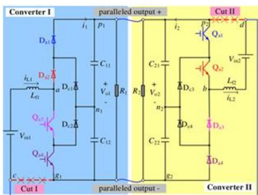
**Fig. 3. Synthesized process of the hybrid boost three-level dc-dc converter by the mode of inputs in series and outputs in parallel.**
