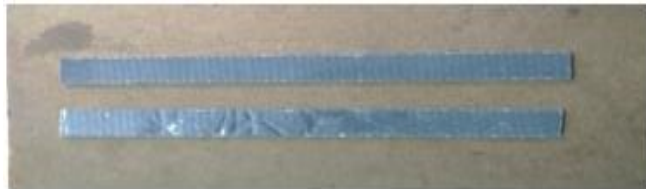
Fig 6.9 Laminate of glass fiber reinforced with aluminum.
