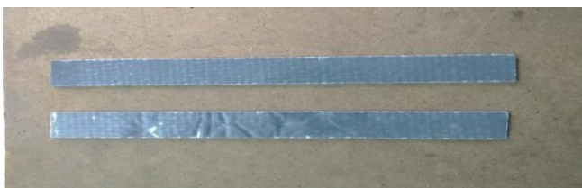
Fig 7.3 Specimen of glass fiber reinforced with aluminium
