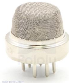
Figure-10 Smoke Sensor
