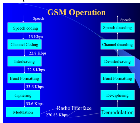
Figure-8 GSM Operation
