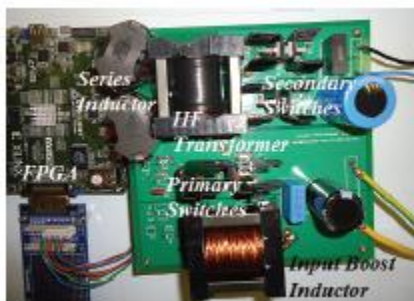
Fig.9. Photograph of the laboratory prototype.
